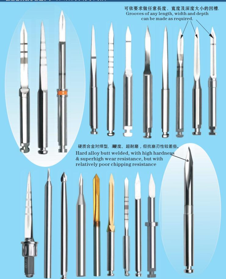
★可超硬、超精研磨、任意的柄部類型、芯厚、容屑槽寬度、刃背方式、鑽尖方式、内冷却孔方式、刃部結構、刃口角度、刃口鋒利程度之要求、及高可至±0.003mm(3μm)的尺寸公差要求 We can produce with super hard and super finish grinding and satisfy your requirement of any type of shank, web thickness, width of chip flute, land, drill tip,inner cooling hole, structure of cutting edge, angle of cutting edge, degree of sharpness of cutting edge, and the dimension tolerance can be up to ±0.003mm(3μm) 💋 LZQ
