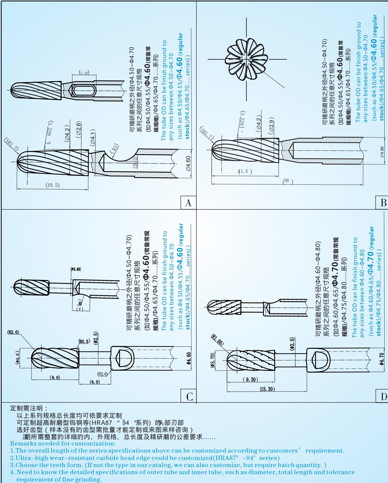
★.依圖依照尺寸/公差/要求複合成型加工，可生產極為複雜、精密的柄部形狀。Compound contour machining according to the sizes/tolerances/requirements of drawings and samples, we can produce extreme complex and accurate holder profile.
