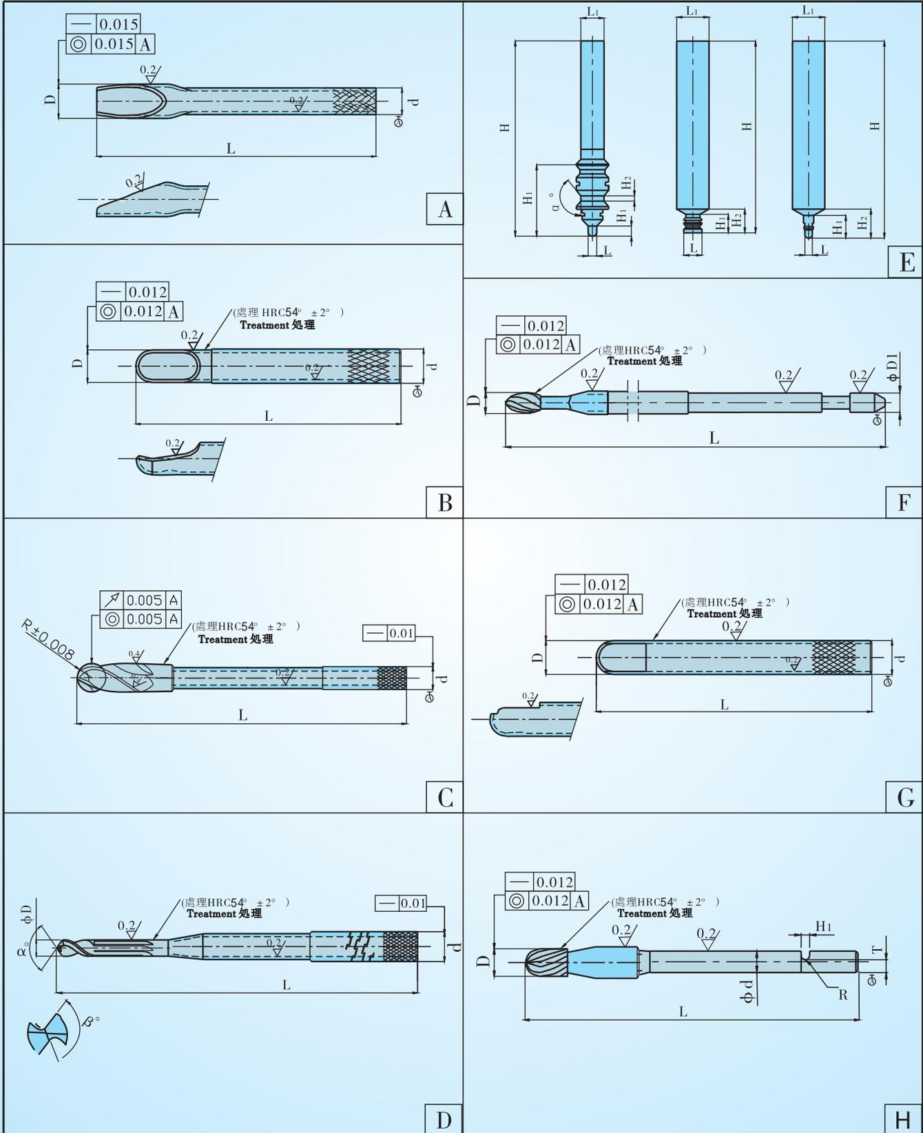
★ 依圖依樣尺寸/公差/要求復合成型加工, 可生產極為複雜、精密的柄部形狀。Compound contour machining according to the sizes/tolerances/requirements of drawings and samples, we can produce extreme complex and accurate holder profile.
